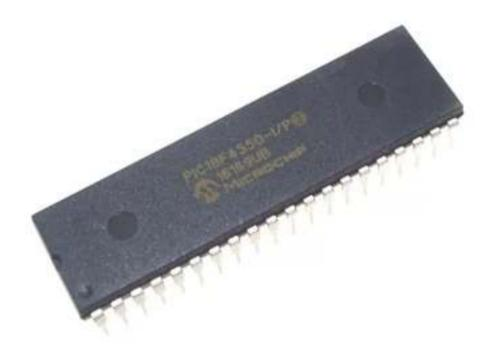
This is an 8-bit microcontroller popular among makers and engineers due its features and easy applications. PIC18F4550 comes in various packages like DIP, QPF and QPN and can be selected according to the project requirement.
