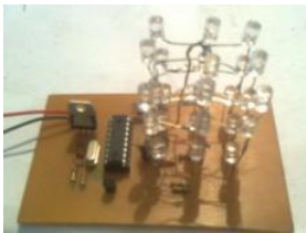
3X3X3 LED CUBE WITH PIC16F628 MICROCONTROLLER CIRCUIT The market plenty of 4 x 4 x 4 led cube was made. I have made 3 x 3 x 3 led cube we also differ. Led cube in each...
