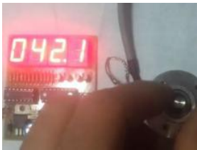
ENCODER, ANGLE MEASUREMENT CCS C PIC16F628 SAMPLE APPLICATION Hi Friends, In this article I will mention the use of incremental enkoderlerin. These encoders with precisely how to angle measurement or position determination to do it. Market the Absolute...
