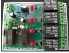
CM8870 REMOTE DEVICE CONTROL VIA TELEPHONE DTMF PIC16F628 PIC16F628 microcontroller and DTMF CM8870 integrated circuits based on the 1, 2, 4 relay has versions with PCB printed circuit drawings are proteus software prepared by the Picbasic. Source code,...
