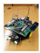
Bluetooth Controlled Robot: This project is used to control robot motion using Bluetooth and android application. Us send control commands from android app to Bluetooth which is connected with pic microcontroller. Microcontroller receives commands from Bluetooth and take respective actions to drive two motor. These..... Listed under: <a href="Bluetoo">Bluetoo</a> Projects
