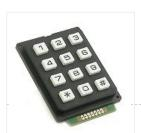
This tutorial explains 'What is a Matrix Keypad?' and 'How to Interface Matrix Keypad with PIC Microcontroller?' Matrix Keypad Matrix Keypad is a very useful and userfriendly when we want to design certain applications like Calculator, Telephone etc. Matrix Keypad is made by arranging push button..... Listed under: Calculator Projects
