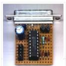
This Programmer is powered by the RS-232 and it works with RS-232 levels at only < ±8.6V. It programs PIC12C5XX, 12C67X, 24CXX, 16C55X, 16C61, 16C62X, 16C71, 16C71X, 16C8X, 16F8X and ISO-CARD's with ASF. Other serial programmable chips by adapter. The high Vpp is obtained by..... Listed under: <a href="Development Board - Kits Projects">Development</a> Board - Kits Projects
