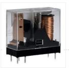
A relay is an electromagnetic switch which is used to switch High Voltage/Current using Low power circuits. Relay isolates low power circuits from high power circuits. It is activated by energizing a coil wounded on a soft iron core. For detailed working of relay please..... Listed under: Other Projects
