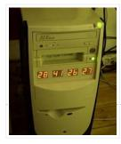
Since I started my watercooling prejoect, I have been verry interested in how well it perform, the only way is to measure all temperatures before and after, The motherboard temperature sensors is useless unacurate, so I'm using LM50B By using this LM50B sensor I get..... Listed under: <a href="How To - DIY - Projects">How To - DIY - Projects</a>, <a href="Projects">Projects</a>, <a href="Projects">Projects</a>, <a href="Temperature Measurement Projects">Temperature Measurement Projects</a>
