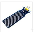
The objective of this project is to design an automatic water level control system. It indicates the level of water in the tank and automatically controls it by using PIC Microcontroller and water level sensors. Water Sensor [caption id="attachment\_15251" align="aligncenter" width="500"] Water Sensor[/caption] Water level...... Listed under:
