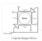
This topic shows how to drive 5V unipolar stepper motor in 3 modes one-phase, two-phase and half step. The microcontroller used in this project is Microchip PIC12F1822 and the motor drive circuit is ULN2003. Usually the unipolar stepper motor has 5 wires one for motor..... Listed under: Motor Projects
