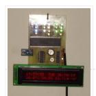
Here we have a clock. It's not "another clock". It has digital and binary output. It also has a thermometer and a hygrometer. It's not "another thermo-hygrometer". It display's absolutely humidity (gr/m3) also. Schematic MCU I build it around Microchip PIC16F917, with internal Oscillator...... Listed under: Clock — Timer Projects
