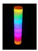
Built utilizing a 24 Channel High Current USB LED Controller to control 12 volt RGB LED Light Strip, in 8 separate groups. Each group has individual 8-bit PWM which can create over 16 million colors. And is driven at full current for maximum color saturation and accuracy. Using...... Listed under: <u>LED Projects</u>
