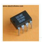
DS1307 is a low power serial real time clock with full binary coded decimal (BCD) clock/calendar plus 56 bytes of NV SRAM (Non Volatile Static Random Access Memory). Data and Address are transferred serially through a bidirectional I2C bus. The RTC provides year, month, date, hour, minute and..... Listed under: <a href="Clock - Timer">Clock - Timer</a>
