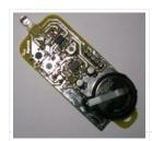
Description The Tiny Remoteis a very compact infrared remote control with only two buttons to control an iRobot Roomba. It produces three different infrared control signals that the robot interprets as Clean, Spot and Virtual Wall/Lighthouse. The circuit is built mostly using SMD components to..... Listed under: <a href="Projects">Projects</a>, <a href="Robotics">Robotics</a> – <a href="Automation Projects">Automation Projects</a>
