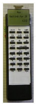
NEC-SIRCS-JAPAN-RC5-SAMSUNG compatible, multiprotocol infrared remote control. Replaces up to 6 existing remote controls into one. With manual learning function, LED display and/or LCD. 2V6-3V2, low power (sleep function) More protocols will be added later if needed (DENON, DAEWOO, MOTOROLA, RECS80.) Components: PIC16LF877-04/L (4Mhz PLCC Package),..... Listed under: <a href="Internet - LAN Projects">Internet - LAN Projects</a>, Projects, Sensor - Transducer - Detector Projects
