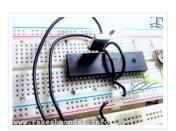
In the simple tutorial we are going to blink few simple led with PIC18F microcontroller, using an external 20MHz crystal oscillator and the '\_Delay ()' function of XC8 Compiler. Most...
