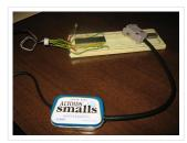
Minty JDM PIC Programmer This project details how to build a JDM style programmer to program PIC Microcontrollers using Microchip's ICSP (In Circuit Serial Programming) and freeware software (PICPgm). Total...
