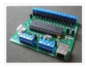
24 Channel USB Connected LED Controller, upto 1A per Channel This device is designed to be a versatile high-current LED controller, with the ability to sink or/and source currents up...
