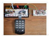
I2C keypad This instructable explains how to interface with a 4×4 keypad over an I2C bus. I started this project because I wanted some plug and play input and output...
