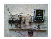
(Some knowledge about RC-5 protocol is required) This project shows how to build a remote controlled real time clock with TFT display using PIC18F4550 microcontroller. In this project DS1307 RTC...
