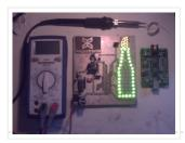
Create your own Beer Bottle LED Volume Unit Meter! This instructable will show you how to create a LED beer bottle VU Meter. A volume unit meter is a device...
