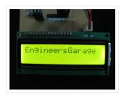
The 16×2 character LCD can work in two modes, namely, 8-bit and 4-bit. These modes basically correspond to the number of data pins used in interfacing LCD. 8-bit mode uses...
