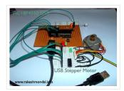
USB Stepper Motor Driver In this project we are going to drive a unipolar Stepper motor (5 wire) using USB interface from a PC Computer. This project is an application...
