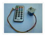
This project shows how to control a 5V unipolar stepper motor from IR remote control uses NEC protocol with PIC18F4550 microcontroller. This controller controls the stepper motor speed and direction...
