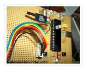
PIC18F4550 USB DEMO INTERFACE BOARD PROJECT This project / USB hardware is quiet easy to make at home with few components, this piece of hardware will be detected by your...
