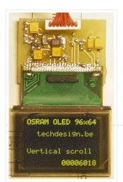
Here are the technical specifications: OLED resolution: 96 x 64 pixels OLED manufacturer: OSRAM. OLED model: Pictiva 1.1 inch OS096064PN11MY0B10 (San Diego.) On-board lcd controller SSD1303, with 31 pins connector....
