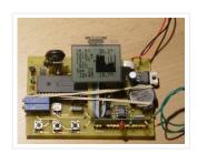
Weather station with pressure reading, relative humidity, indoor & remote outdoor temperature display. Both Celsius or Fahrenheit & mbar/hPa or mm Hg supported. With calendar & clock. Easy 3-button user-menu....
