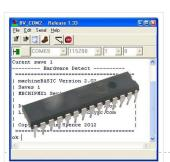
\$15.00 BASIC Computer? Imagine a microcontroller that you can connect a serial terminal up to to get an ok prompt? What would happen if you changed one of the control...
