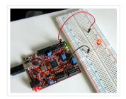
The PIC32 processor on the chipKIT Uno32 board provides two hardware serial ports. One of these is used by the on-board FTDI chip to create an USB-UART interface that allows...
