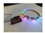
There has not been a simple addressable LED library for PIC32 microcontrollers until now! The PICxel library is an MPIDE library that handles the timing required to use addressable LEDs...
