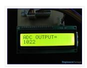
This post provides the ADC code using PIC16F877 microcontroller. This code is written in C language using MPLAB with HI-TECH C compiler. You can download this code from the 'Downloads' section at...
