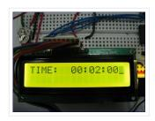
A Digital Clock can be made easily by using PIC Microcontroller, DS1307 and a 16\*2 LCD. I have already posted about Interfacing DS1307 RTC with PIC Microcontroller. The DS1307 RTC...
