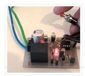
Project Summary Build yourself a single shot Pic Micro Controlled by stable Relay FEATURES 1. One touch activated for on or off 2. Open connections for other sensors 3. 10...
