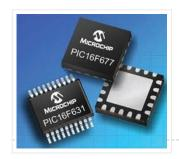
Peripheral Interface controller (PIC) family is one of the most powerful advanced microcontroller which is developed by the microchip technology with Harvard architecture, i.e., it has a minimum set of...
