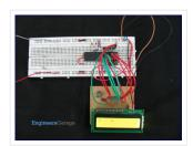
This post provides the LCD[1] interfacing code in 4bit mode using PIC16F84A microcontroller. This code is written in C language using MPLAB with HI-TECH C compiler. You can download this code from the 'Downloads' section at...
