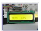
OBJECTIVE: Temperature measurement Digital display of temperature used of microcontroller to measure temperature used of microcontroller to Display temperature value on LCD (liquid crystal display) Components: There are many temperature...
