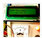
This post provides a simple digital voltmeter circuit using PIC12F675 microcontroller. This code is written in C language using MPLAB with HI-TECH C compiler. You can download this code from the...
