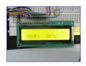
Thermometer can be easily constructed using a PIC Microcontroller and LM35 Temperature Sensor. LM35 series is a low cost and precision Integrated Circuit Temperature Sensor whose output voltage is proportional...
