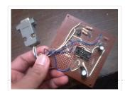
In this instructable, I'll show you how I built and tested this simple yet powerful circuit. The JDM Programmer is my favorite Microcontroller programmer. It is a...
