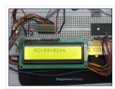
This post provides a simple digital clock implementation using PIC16F84A microcontroller and an LCD display. This code is written in C language using MPLAB with HI-TECH C compiler. You can download...
