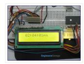
This PIC16F877 microcontroller tutorial answers the question, "How to implement a digital clock using PIC16F877?" Using PIC16 simulator (Proteus) you can verify this digital clock code and...
