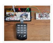
This post provides a simple method to interface any keypad (e-g 4×4 or 4×3 etc) with PIC12F675 microcontroller. The code for PIC12F675 is written in C language using MPLAB with HI-TECH...
