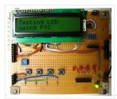
This post provides the LCD[1] interfacing code using only 3 pins of PIC16F84A microcontroller. This code is written in C language using MPLAB with HI-TECH C compiler. You can download this...
