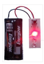
Description This project is a multi-function LED bike (cycle) light using 3 LEDs. It is based on a PIC10F200 baseline microcontroller, running from a supply voltage of 2 to 5...
