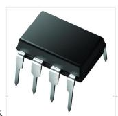
This post provides the code for interfacing 24LC64 EEPROM with PIC16F877 microcontroller. This 24LC64 EEPROM has i2c based interface. This code is written in C language using MPLAB with HI-TECH C...
