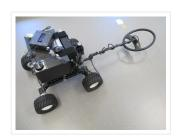
Metal detector robot using pic microcontroller, this robot is designed for metal detection in places where human being can't reach easily. Metal dectector robot detect metal through metal detector sensor. Its...
