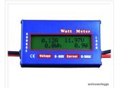
Digital dc watt meter using pic microcontroller is used to measure dc power of dc circuits. Voltage and current sensors are used in this project. Voltage and current sensors are...
