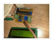
Digital Ammeter circuit using pic microcontroller is designed to measure dc current. In this project, you will learn how to measure dc current using pic microcontroller? how to convert current...
