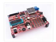
Development board backplane Plug-in part by wave soldering process, the board also neat reverse. The curved surface of the pad foot, guaranteed not to scratch your desktop....
